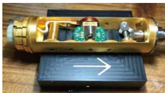
Fig. 2 Photograph of a miniature pressure cell placed on the horizontal rotator for PPMS
